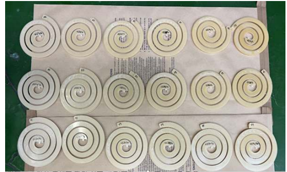
Spiral flow length (2t, nozzle 240°C, mold 80°C) - M93FE2Y: initial length is 900mm, and over 95% flow length retention after 30min dwelling
