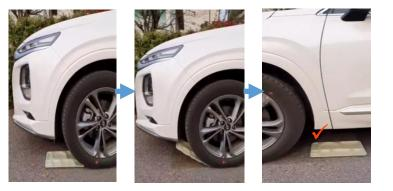
[POKETONE molded part of food tray Never Deformed after vehicle load]
