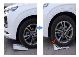
[Melamine food tray Completely Cracked after vehicle load]
